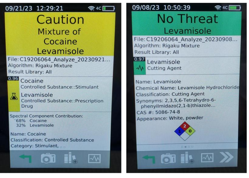
**Figure 2.** Example of the color-coded results from the ResQ-CQL internal library identification system when detecting a potentially harmful substance (left) and a non-threat (right).
