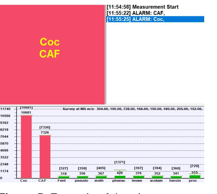
Figure 5. Example of the alarm system detecting a mixture of caffeine and cocaine on the Continuity instrument. The mass spectra are searched against the user-defined library.
